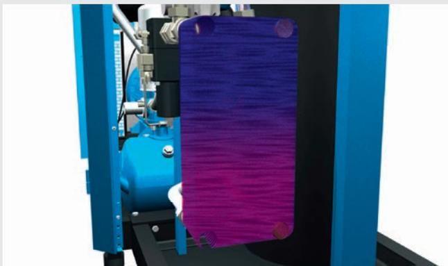
1. The compressed air is pre-heated to 200°C.
