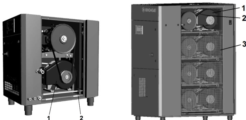
Fig. 6.8: View of the right side of the EO 6 (left) and EO 11...22 scroll unit housing
