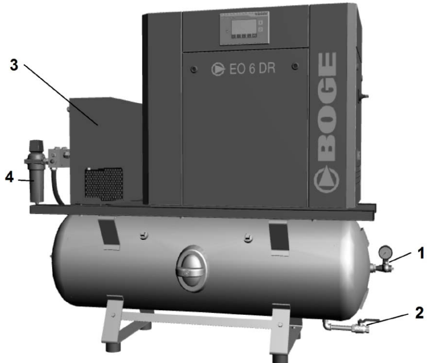
Fig. 6.2: Overview of additional maintenance work on the compressor unit or station
