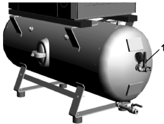
Fig. 3.3: Safety valve (1) on receiver EO 6 R
