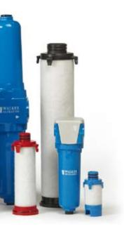
Every 1 barg (100kPa) of pressure drop represents a 7% increase in compressor energy costs. It is vital to observe a scheduled maintenance programme which includes replacement of filter elements.
