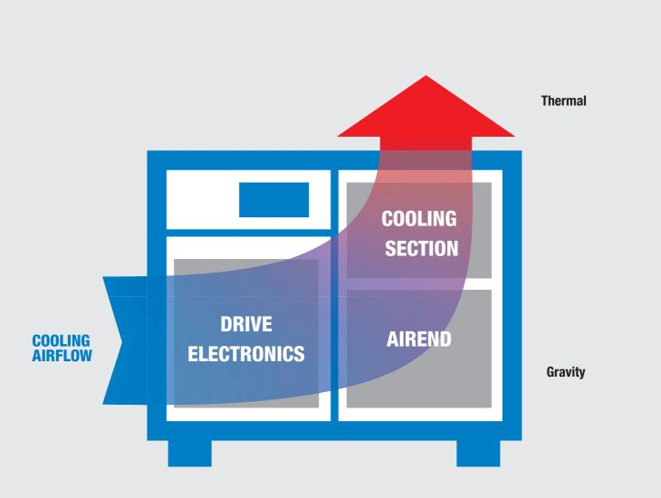
Intelligent engineering from BOGE: The three main sections of the BOGE screw compressor (electrics & drive, compressor, independent cooling unit) are strategically aligned in the main cooling air flow: for maximum efficiency and service life.
